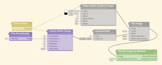
**Count within Range** is one of many ways to cycle through a series of numbers. Another is the **Curve** node when its **Loop** port is set to *Loop* or *Mirror*. And another is the **Wave** node. The composition below (File) Open Example vuo.motion Wave Circle) uses the **Wave** node to make a circle move back and forth.
