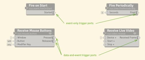
Each event is fired from a **trigger port**, a special kind of output port on a node.
