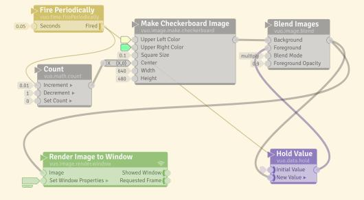
This works. An event from the **Fire Periodically** node travels through the **Count** node to the **Make Checkerboard Image** node, to the **Blend Images Node**. The same event travels through a separate cable to the **Hold Value** node, and then to the **Blend Images** node. There the two events are joined.
