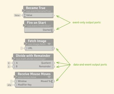
**4.2.2.1 Trigger ports** Although trigger ports can *create* events, they never *transmit* events that came into the node through an input port (hence the thick line to the left of each trigger port — an event wall), nor do they cause any other output ports to emit events.
