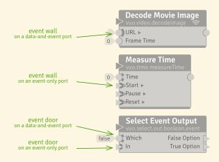
Ports that always block events have a solid semi-circle (like the **URL** port above) or a solid chevron (like the **Start** port above). This is called an **event wall**. The node must receive an event from another port without an event wall for the results of the node's execution to be available to other nodes.
