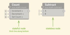
Some nodes have **state**. A **stateful node** retains information from the last time it executed. An example of a stateful node is **Count**. If a **Count** node is told to increment, its state (the retained count) changes.
