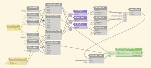
Here's one more example. It demonstrates how conditions can be used to coordinate between nodes downstream of different triggers. The composition displays the message "Camera detected" once it starts receiving input from the user's video camera, that is, once the **Receive Live Video** node's trigger
