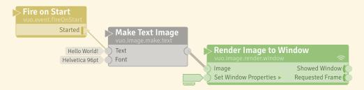
In the above composition, the **Text** input port of the **Make Text Image** node inputs an event, which causes the node to execute. The **Image** input port of the **Render Image to Window** node inputs the event and an image. When the node executes, it uses that image to do its job of rendering an image to a window.
