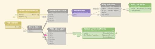
**Became True** node outputs an event each time the output of **Is Within Rectangle** changes from *false* to *true*, emitting a sound effect each time the mouse cursor enters the square.
