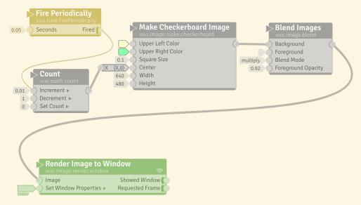
But you want to see the effect of taking the produced image from the **Blend Images** node and feeding it back into the **Foreground** input port of the node. If you try that, you see that you create an infinite feedback loop, because there is no event wall on the **Foreground** input port to stop an event from entering the node a second time.
