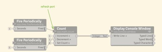
For example, the composition above shows how you can use the refresh port to get the **Count** node's current count without incrementing or decrementing it. When the lower **Fire Periodically** node fires an event, **Display Console Window** writes the incremented count. When the upper **Fire Periodically** node – which is connected to the **Count** node's refresh port – fires an event, the count stays the same. **Display Console Window** writes the same count as before.
