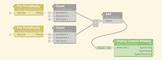
In this composition, the **Add** node executes each time either **Fire Periodically** node fires an event. If one of the **Add** node's inputs receives an event, it doesn't wait for the other input. It goes ahead and executes.
