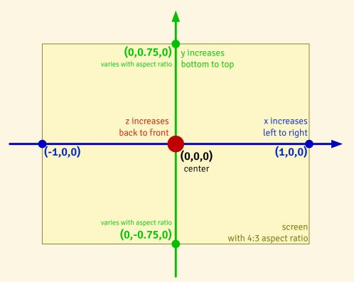
Typically, as illustrated above, the position (0,0) for 2D graphics or (0,0,0) for 3D graphics is at the center of the rendering area. The X-coordinate -1 is along the left edge of the rendering area, and the X-coordinate 1 is along the right edge. The rendering area's height depends on the aspect ratio of the graphics being rendered, with the Y-coordinate increasing from bottom to top. In 3D graphics, the Z-coordinate increases from back to front.
