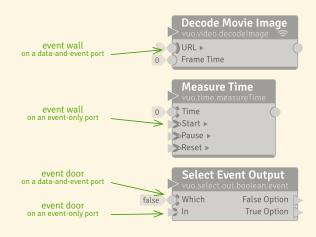
The composition below, Select Movie (File Open Example vuo.select), demonstrates one way that event doors can be useful. This composition displays one of two movies at a time, switching between them each time the mouse is pressed. The doors on the **Select Input** node's **False Option** and **True Option** input ports allow the node to let the stream of events and video frames from one movie through while blocking the stream from the other movie.
