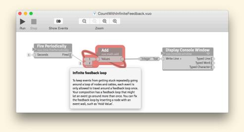
The above composition is an example of an infinite feedback loop. Any event from the **Fire Periodically** node would get stuck forever traveling in the feedback loop from the **Add** node's **Sum** port back to the **Item 1** port. Because there's no event wall in the feedback loop, there's nothing to stop the event. Every feedback loop needs a node like **Hold Value** to block events from looping infinitely.
