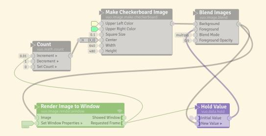
In this case, you can use the same stream of events into the **Count's Increment** port, simplifying your composition. Using events from a **Rendered Frame** trigger port is usually the best way to provide events for any type of animation in your composition.
